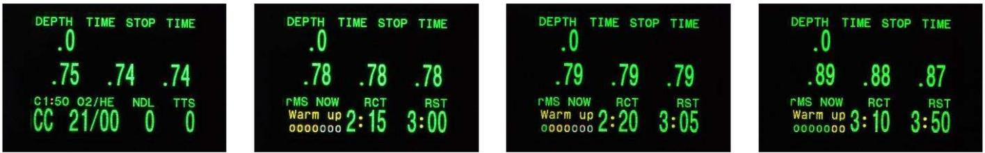
Also on the main screen there is an indication if the scrubber is fully ready or not: as long as the warming up is not yet finished, the colon between the C and the number is yellow, and only when the scrubber is fully warmed and ready, the colon becomes green, and full information of the total scrubber can be used to predict the cycle and scrubber times.
