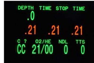
If you don't see 'C ?' this means that your temperature probes are switched off in the 'System Setup'. Go to the setup menu and change the setting of the temperature probes to 'on'. Switching 'off' the temperature probes can be done when diving on the dual radial scrubbers, or when using classic non-rMS axial scrubbers.
