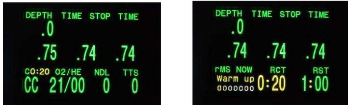
With only the temperature info at the inlet of the scrubber, the system has already received enough data to predict a minimum remaining time. You can see on the info screen that the warming up of the first zone in the scrubber has started: the color changed to yellow. However, only when that zone is fully warm, the color will be come green.
