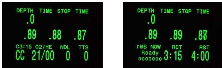
From this point on, and in dive mode, the minimum remaining cycle and scrubber time of the dive is logged, while at the same time the actual RCT/RST is shown on the main screen and the extra info screen.
