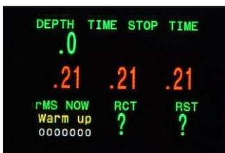
This screen shows that the unit is ready for warm up, but none of the 7 zone's have started to become active (they are all grey) so no prediction can be made for RCT or RST
